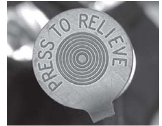
bottom of RIC charging hose
