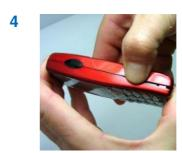
Hold front of phone firmly whilst freeing the back cover, then pull the back cover away from the very bottom of the phone.
