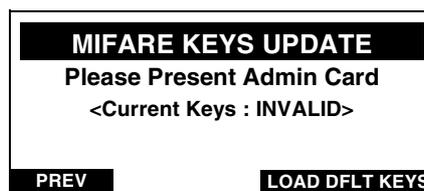
Pressing the **LOAD DFLT KEYS** hotkey will allow you to re-update the 32 keys with the default value 0xFFFFFFFF.
