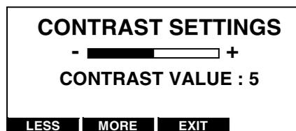
The **CONTRA** selection allows you to adjust the contrast of the LCD display.
