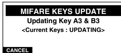
When the MorphoAccess™ finishes to update the keys for the 16 sectors, a successful message appears. The keys status indicates now "user" keys, meaning keys different from 0xFFFFFFFF have been loaded into the reader. Then the MorphoAccess™ comes back to the administrator menu after 2 seconds.
