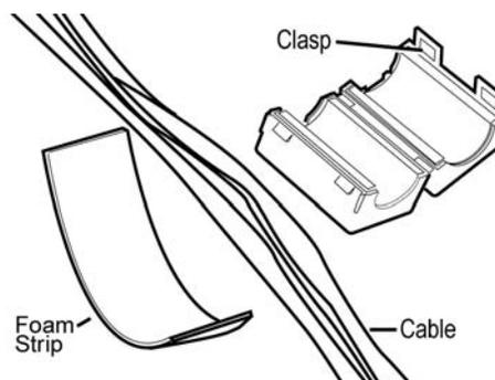
1. Open a ferrite bead by releasing the clasp on the side.
