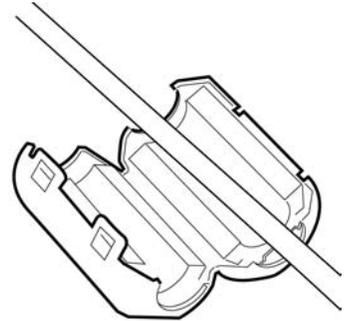
3. Bend the cable around the ferrite bead to form a loop and lay it again inside the ferrite bead.
