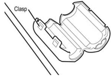
2. Position the ferrite bead on the cable as close as possible to (but not inside) the MorphoAccess.
