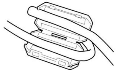
4. Close the two halves of the ferrite bead and securely fasten the clasps without pinching the cables.
