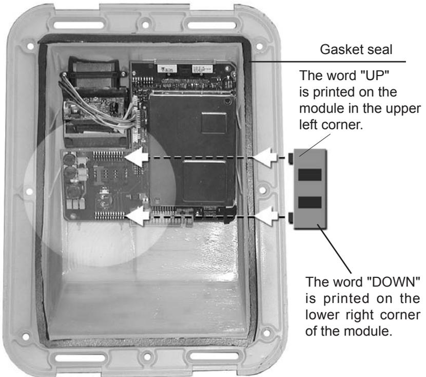
5. Use approved static discharge protection. Remove the memory module from its protective ESD packaging.
