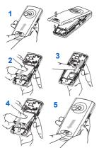
The SIM card is inserted under the phone's battery. Ensure that the phone is switched off and the charger disconnected.
