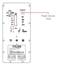
Once powered on rotate the speaker's Master Volume Knob to the right to increase the master volume or to the left to decrease the master volume.
