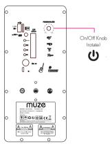
1. Rotate the ON/OFF Knob to the right in order to power on your speaker. Rotate it all the way to the left to power off your speaker.
