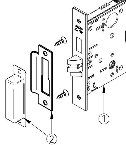
Recommendation for Customer's lever set installation on SALTO AELEMENT.
