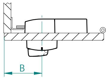
(Eng) The dimension B will depend on the door or strike type the locker lock is going to be installed on.
