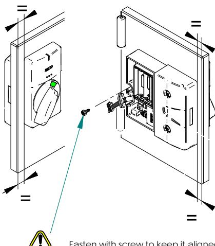
Fasten with screw to keep it aligned.
