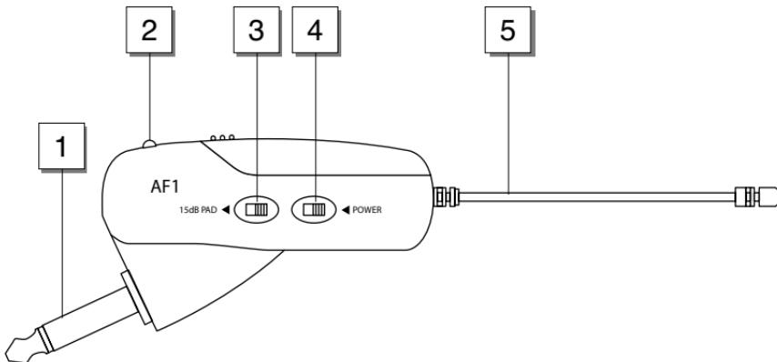
**Note:** The AF1 and AG1 transmitters are functionally identical apart from the angling of the 1/4" plug. For purposes of illustration, only the AF1 is shown on these pages.
