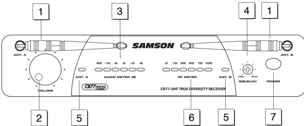
**2: Volume control** - This knob sets the level of the audio signal being output through both the balanced and unbalanced output jacks on the rear panel (see #2 and #4 on page 9 in this manual). Reference level is obtained when the knob is turned fully clockwise (to its "10" setting).
