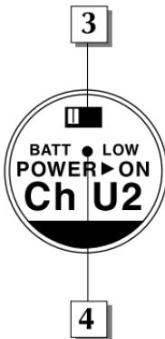
**4: Power / Battery LED** - This LED flashes once when the AX1 is first turned on and lights steadily red when there is less than 2 hours of battery power remaining, indicating that the battery needs to be changed.
