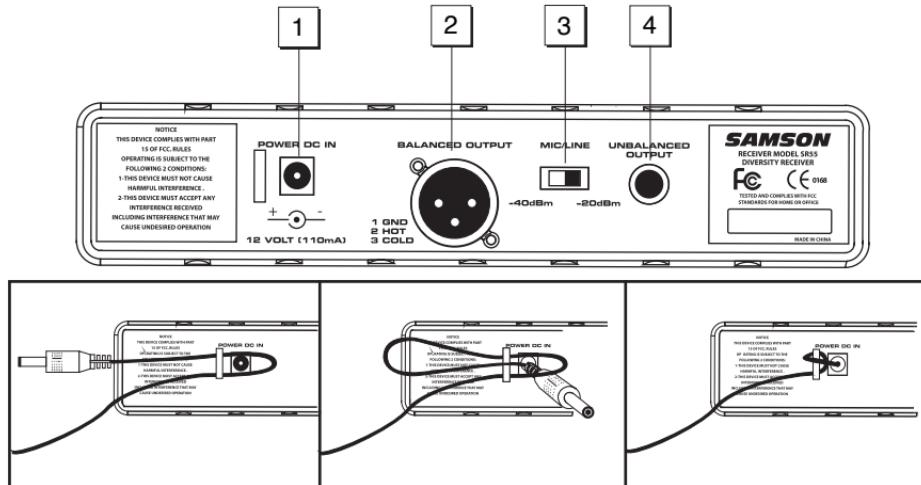
**Using the strain relief:** Gather up a loop of wire and pass it through the strain relief, then pass the adapter plug through the loop in order to create a knot.
