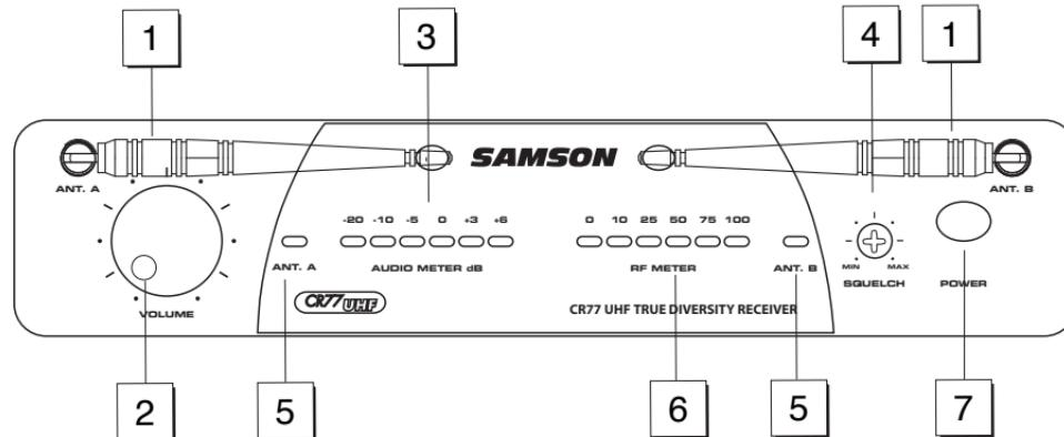
**1: Antennas (A and B)** - The antenna mountings allow full rotation for optimum placement. In normal operation, both Antenna A (the antenna on the left) and Antenna B (the antenna on the right) should be placed in a vertical position. Both antennas can be folded inward for convenience when transporting the CR77. See the "Setting Up and Using the AirLine System" section on page 17 in this manual for information about antenna installation and positioning.
