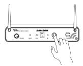
Turn on the power to the transmitter by pressing and holding the Power switch; the indicator LED will light green.
