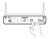
Position the transmitter about 6-12" (15-30 cm) from the front of the CR88 with the transmitter's IR window facing the IR transmitter on the front panel of the CR88 receiver.
