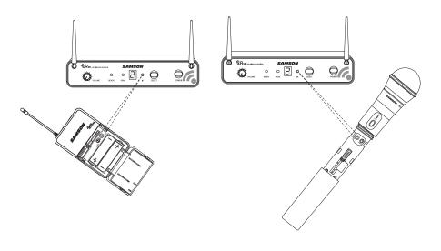
When the transmission is complete, and the CR88 is receiving RF signal from the transmitter, the READY indicator will light on the front panel of the CR88 receiver.
