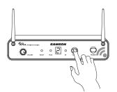
Press and hold the CR88 SELECT button to set the transmitter to the same channel as the receiver via infrared transmission
