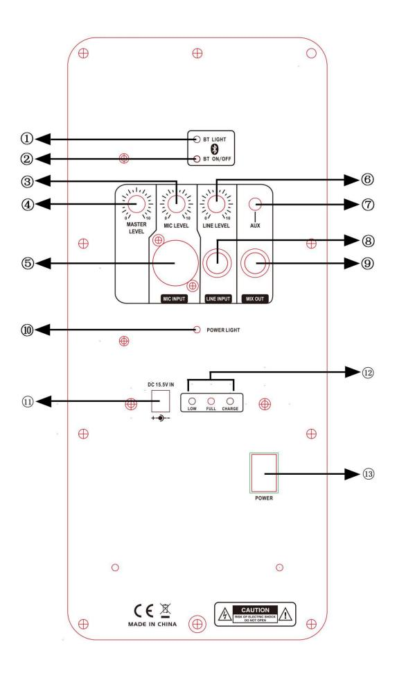
**1.BT LIGHT:**When the light flashes, can connect to BT.Stop flashing indicates that it is connected.
