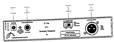
1: DC Input - Connect the supplied 12 volt 160 mA power adapter here, using the strain relief as shown in the illustration below. WARNING: The substitution of any other kind of power adapter can cause severe damage to the SR44 and will void your warranty.
