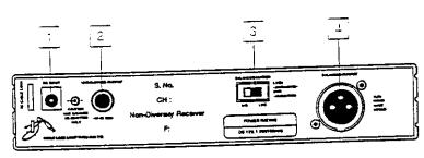
1: DC input - Connect the supplied 12 volt 160 mA power adapter here, using the strain relief as shown in the illustration below. WARNING: The substitution of any other kind of power adapter can cause severe damage to the SR4 and will void your warranty.
