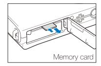
Push gently until the card disengages from the camera and then pull it out of the slot.
