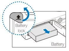
Push the lock up to release the battery.
