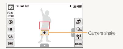
When shooting in the dark, avoid setting the flash option to **Slow Sync** or **Off**. The aperture remains open longer and it may be harder to hold the camera still.
