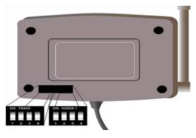
and receiver channel switch. At the bottom of receiver are there mouse and keyboard channel. The receiver is as shown in the following.
