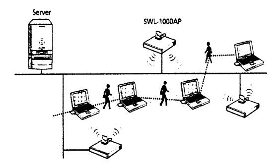
Roaming is a service that disconnects the user from an access point allotted to the previous cell and connects to the one allotted to a new cell when the user moves into the cell.
