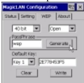
You can generate 40bit or 26bit WEP keys without entering all hex values using the same 'Pass Phrase' between AP and wireless client. After typing pass phrase, click 'Generate' button. Then WEP keys will be generated. This option is used ONLY among MagicLAN products.
