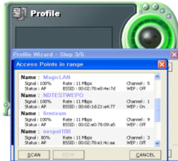
4. If you clicked on the Survey, the above window will appear showing you Access Points or Stations (Ad hoc) that are able to connect now. Select the AP that has the highest signal to use as an SSID.
