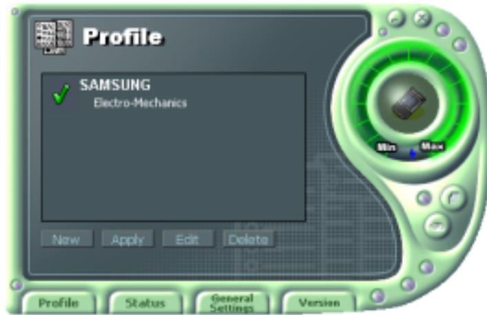
8. Click the Profile name shown in the above window click the Apply button. The settings will be over. If the IP address entered in the system settings is different than the IP address selected under profile name, system IP settings will be changed without rebooting your system.
