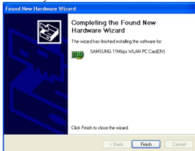
5. Check for the [SAMSUNG 11Mbps WLAN PC Card](#) on **Computer Management** in the **Administrative Tools** of the **Control Panel**. If you find the **Yellow** sign on the adapter, it shows the installation is not successful. In this case, select the adapter and click on **Remove**. Restart your computer after uninstalling the driver to make
