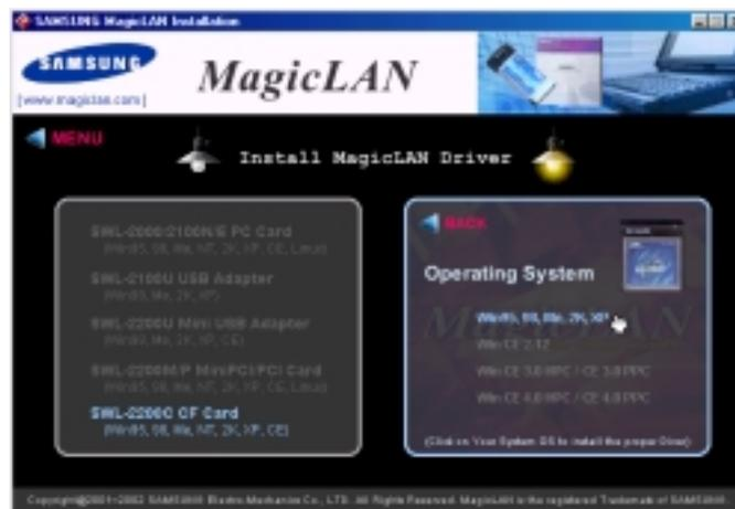
4. After installing driver, insert Wireless LAN card. You can click **Continue Anyway** in the 'Hardware Installation' Message box.
