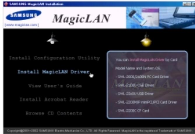
2. You can see the pictures of Wireless LAN Cards by model name.(SWL-2200C CF Card). Click on the model name to install it's driver.
