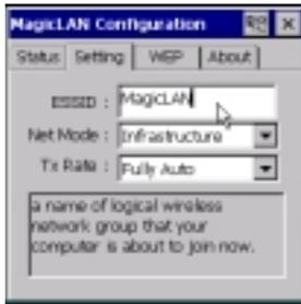
You can change ESSID. Be careful to insert exact ESSID to connect AP or wireless client. Upper and lower characters are distinguishable. If you use 'ANY' or 'any', your system will try to connect to nearby AP or wireless client randomly.
