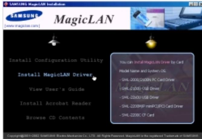
2. You can see the pictures of Wireless LAN Cards by model name.(SWL-2200C CF Card). Click on the model name to install it's driver.
