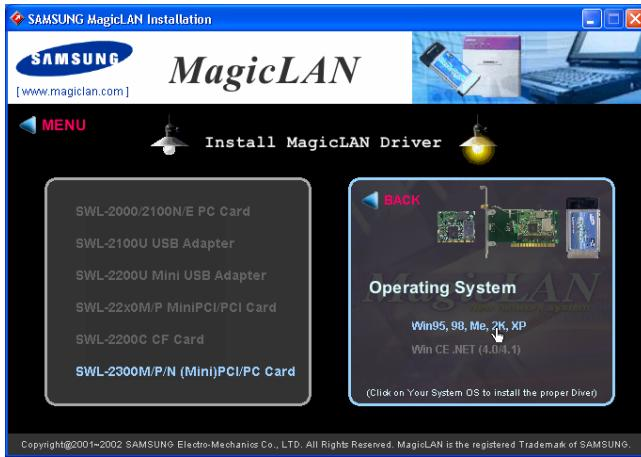
4. After installing driver, click on ‘MENU’ and ‘Install Configuration Utility’ and you can install configuration utility. After installing driver and utility, insert Wireless LAN Card.(notice that in case of PCI product like SWL-2300M/P , you must power off before inserting Wireless LAN Card into the system)
