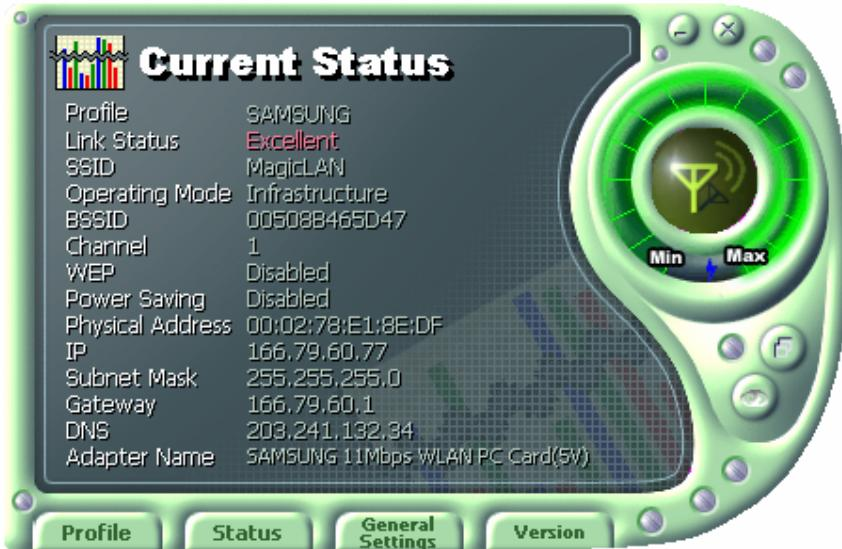
**Profile:** Profile is the name of the current profile that configuration utility is using.
