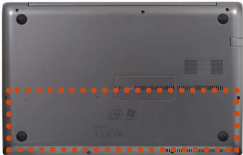
The location of the internal battery
