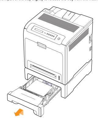
2 If you see the jammed paper, remove the paper from the machine by gently pulling it straight out as shown below.
