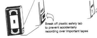
Cover the record protect space with cellophane tape to make a new recording
