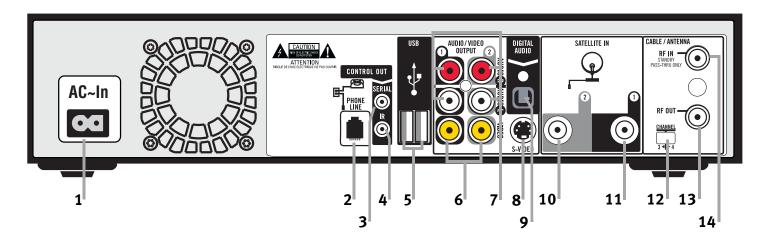
This section describes the use of the connection jacks and switch on the back panel of the DIRECTV® DVR. If your setup doesn't match any of the examples, you can use this information for general reference as you set up your equipment.
