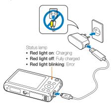
Use only the AC adapter and USB cable supplied with your camera. If you use another AC adapter (such as SAC-48), the camera battery may not charge or work properly.
