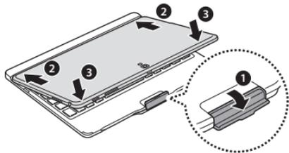
To separate the tablet from the device, completely open the fastener clip, and then pull the tablet upwards.
