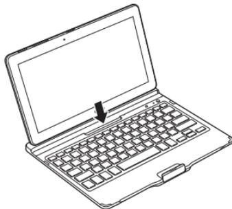
To remove the tablet from device, lift the tablet upwards.
