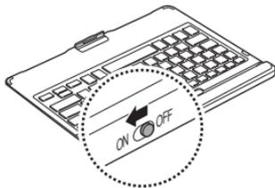
Slide the Power switch to **OFF** to turn off the device.
