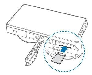
4 Replace the flap and slide the latch.
