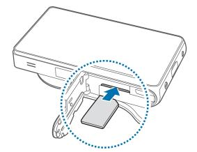
Do not insert a memory card into the SIM card slot. If a memory card happens to be lodged in the SIM card slot, take the device to a Samsung Service Centre to remove the memory card.
