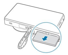
$\boldsymbol{3}$  Push the SIM or USIM card until it disengages from the device, and the pull it out.
