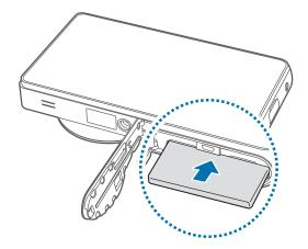
5 Replace the flap and slide the latch.
