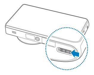
2 Insert the SIM or USIM card with the gold-coloured contacts facing downwards.
