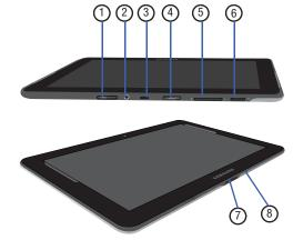
Infrared Blaster: used to emit infrared signals used for controlling external devices. For more information, refer to "Smart Remote" on page 195.
