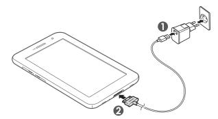
Connecting the USB cable improperly may cause serious damage to the device or USB power adapter. Any damage caused by misuse is not covered by the warranty.
