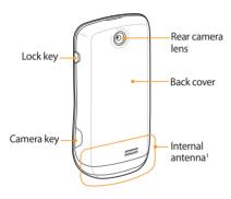
1. Avoid contact with the internal antenna area while the phone is receiving or transmitting signals.
