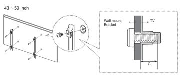
nstall your wall mount on a solid wall perpendicular to the floor. If you are attaching the wall mount to building materials other than plaster board, contact your nearest dealer. If installed on a ceiling or slanted wall, the TV may fall and cause severe
