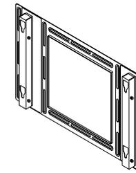
The factory default angle of wall attachment panel is 5 degrees.
