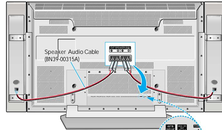
\* External speakers MUST have a power handling capability of 10 watts minimum (impedance 8 ohm).
