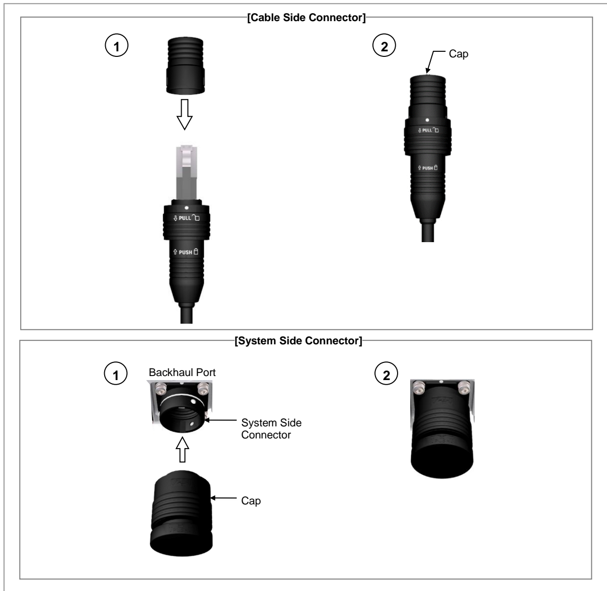
Figure 76. Removing the Interface Copper Cable; Push Pull Type (2)
