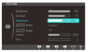
4 Adjust the Sharpness using the [▲/▼] buttons.
