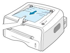
When you pull the jammed paper, if there is resistance and the paper does not move immediately, stop pulling. Continue with the next step.
