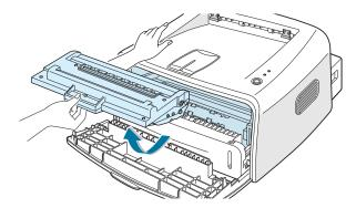
3 With a dry, lint-free cloth, wipe away any dust and spilled toner from the toner cartridge area and the toner cartridge cavity.
