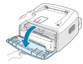
2 Remove the toner cartridge from the printer.
