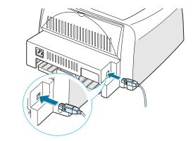
**Note:** If you are using a USB hub, connect the printer's cable to the first tier of the hub, or the printer may malfunction. If the printer doesn't work with the hub, connect it directly to the USB port.
