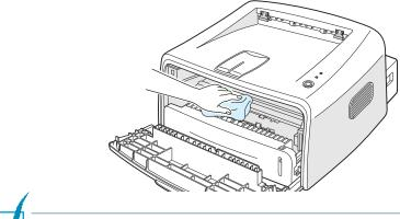
**Note:** To prevent damage to the toner cartridge, do not expose it to light for more than a few minute. Cover it with a piece of paper, if necessary. Also, do not touch the black transfer roller inside the printer.
