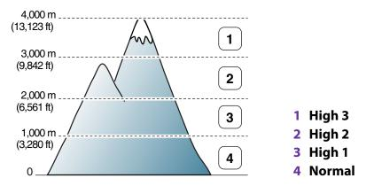
You can set the altitude value from **Device Settings** or **Machine** section in Printer Settings Utlity program.
