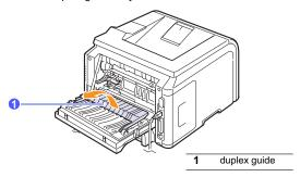
While pushing the fuser lever to the right, open the fuser door.
