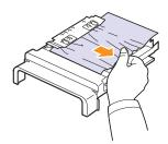
If the paper does not come out with the duplex unit, remove the paper from the bottom of the printer.
