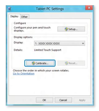
2 Select the screen type to calibrate. If the **Calibration** screen appears, touch the point represented by the "+" mark and then remove your finger.
