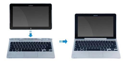
When the keyboard dock and the computer are properly connected, the keyboard dock **power indicator**  $\bigcirc$  is turned on.
