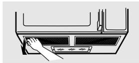
**To remove**, slide it to the outside using the tab. Pull it down and out.
