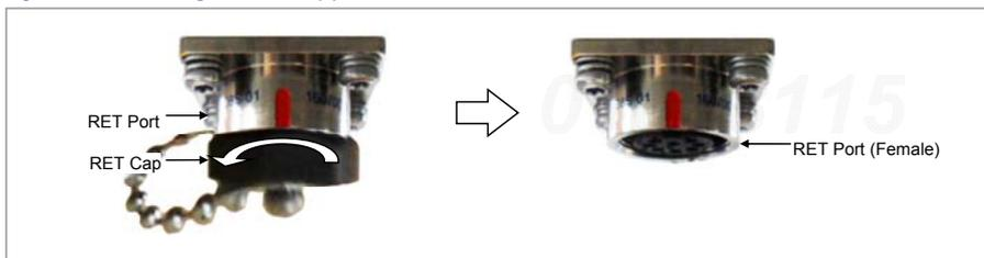
4 Connect the cable side RET connector to the system side RRH RET port.
