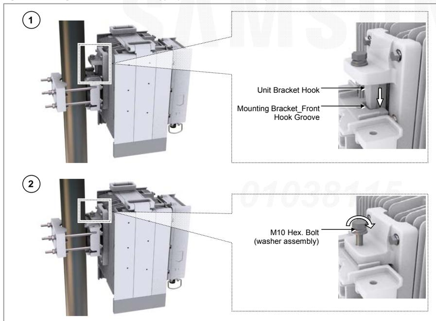
Figure 30. Fixing RRH\_1 Sector Pole Type (Side Installation)
