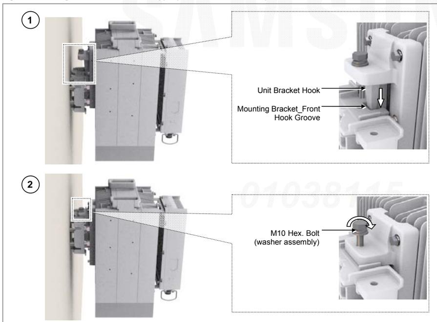
Figure 57. Fixing RRH\_1 Sector Pole Type (Side Installation)
