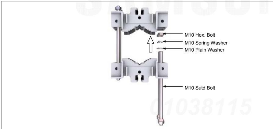
3 Place a mounting bracket assembly to the pole.
