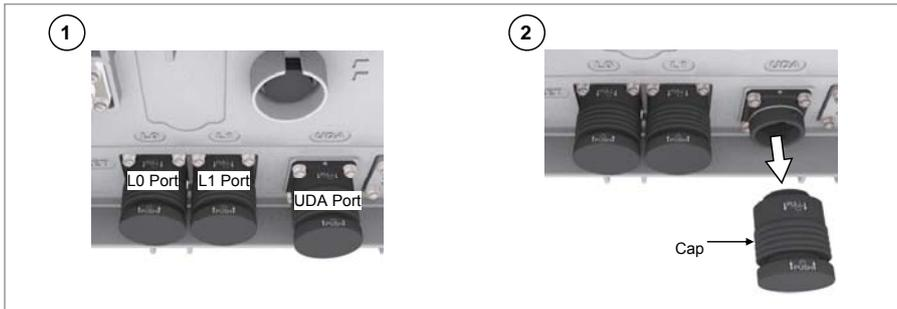
4 Separate the cap from the cable side connector.
