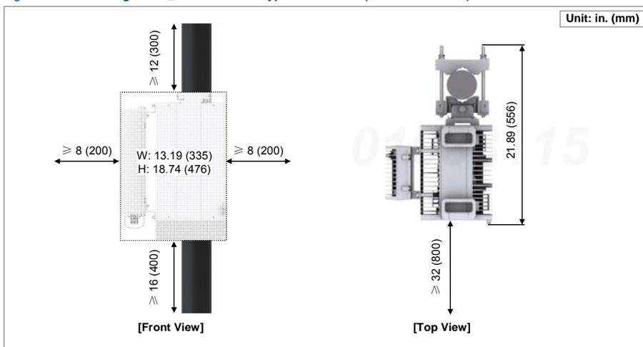
Figure 8. RRH Arrangement\_2 Sector Pole Type Installation (Back to Back Installation)
