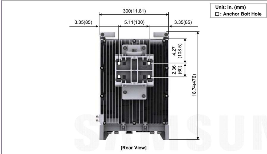
Figure 52. RRH marking dimensions\_1 Sector Wall Type (Side Installation)
