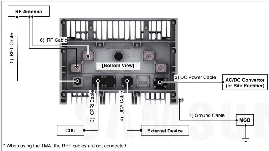
Figure 61. RRH Cable Diagram\_RF Connection: 2T4R, 4T4R
