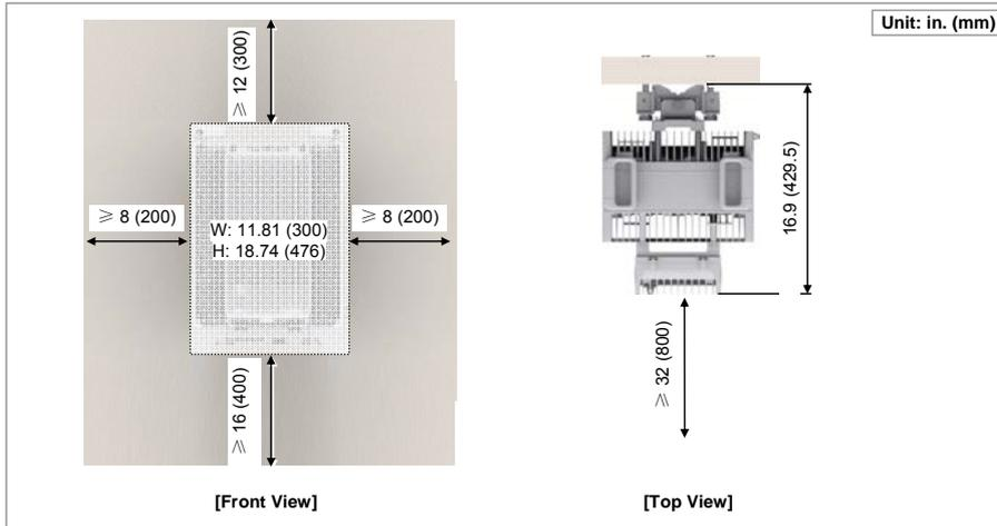
Figure 11. RRH Arrangement\_1 Sector Wall Type Installation (Side Installation)
