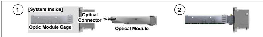
Inset the optical module's bail, facing the front of the system, to the port.
