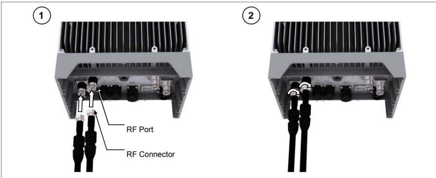
7 After connecting the connector, push waterproofing boots up to the connector connection.
