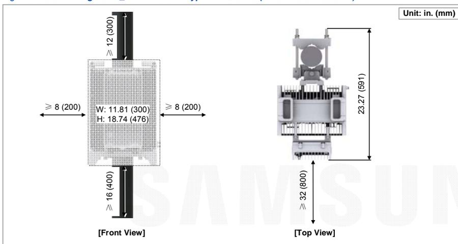
Figure 7. RRH Arrangement\_1 Sector Pole Type Installation (Side Installation)
