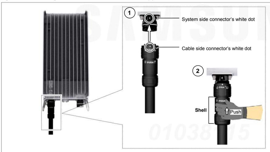
When the connector is fastened tight, the white line on the system side connector should be invisible (or hidden).
