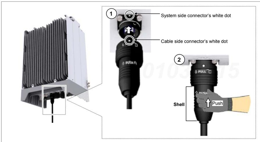
When the connector is fastened tight, the white line on the system side connector should be invisible (or hidden).
