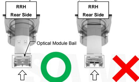
Do not inset when the optical module's bail is unlocked.
