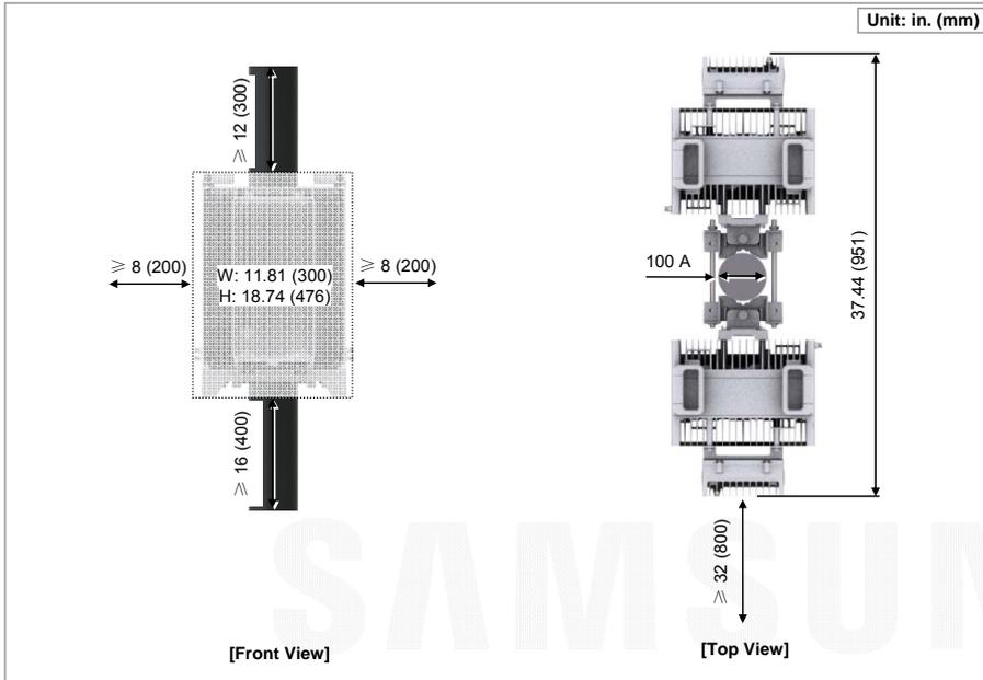
Figure 9. RRH Arrangement\_2 Sector Pole Type Installation (Side by Side Installation)
