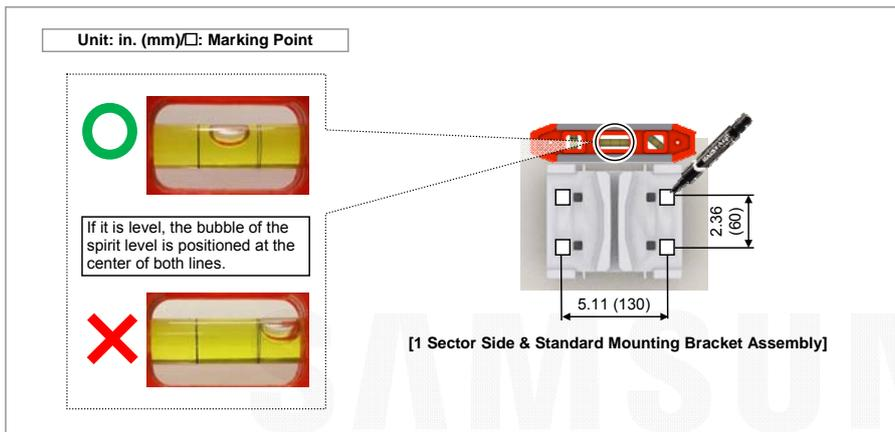
▶ To drill anchor holes and fix anchors
