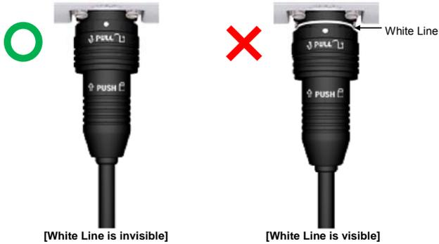
The method for connecting/disconnecting the CPRI (optical) connector is as follows:
