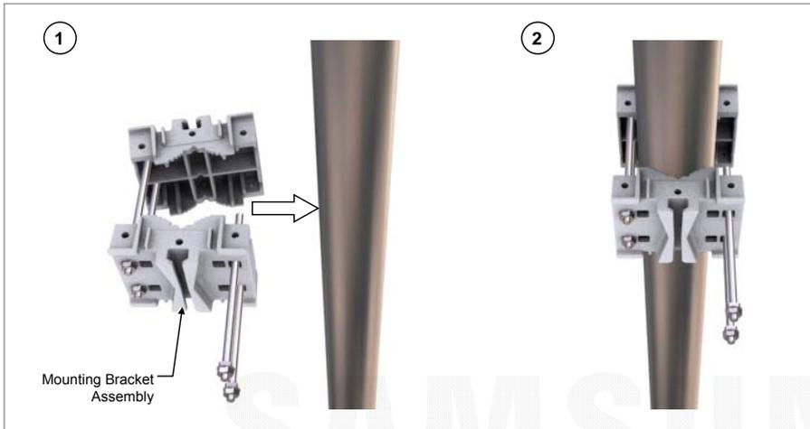
4 Pass a stud bolt through 2sector mounting bracket assembly\_front hole and fix mounting bracket assembly using fasteners.
