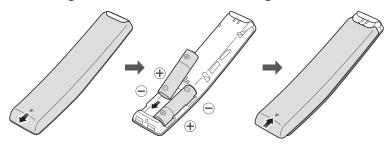
To install the batteries, push the rear cover open in the direction of the arrow at the bottom of the illustration, and then insert the batteries as shown in the figure. Make sure that the positive and negative ends are facing in the correct direction. Close the rear cover as shown.
