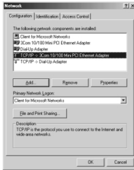
Figure 40. Installing the LAN Driver
