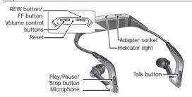
If your headset responds slowly, stops responding, or freezes, press the reset on the back of the headset with a pointed tool.
