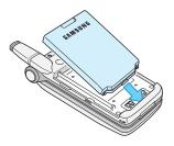
2. Press the battery down until it snaps into place.
