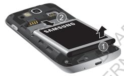
3. Lift the battery up and out of the phone (2)
