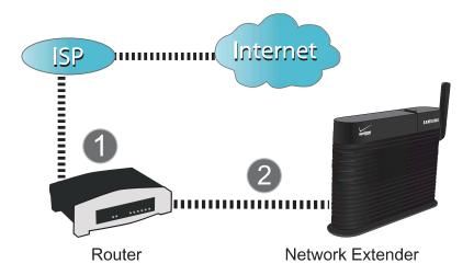
**5.** Connect one end of the included Ethernet cable to an open LAN port on the router (1) and connect the other end to the WAN port located at the rear of the Network Extender (2).
