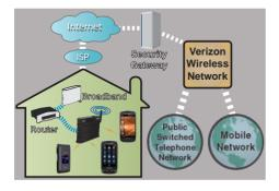
About the size of a traditional wireless access point (WAP), the Network Extender facilitates the delivery of cellular traffic through the Internet to the Verizon Wireless network, which then routes the signal to the desired party.
