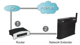
Connect one end of the included Ethernet cable to an open LAN port on the router (1) and connect the other end to the WAN port located at the rear of the Network Extender (2).
