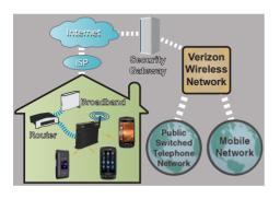
About the size of a traditional wireless access point (WAP), the Network Extender facilitates the delivery of cellular traffic through the Internet to the Verizon Wireless network, which then routes the signal to the desired party.
