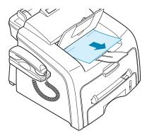
If there is any resistance and the paper does not move when you pull or if you cannot see the paper in the front output tray, continue to step 3.
