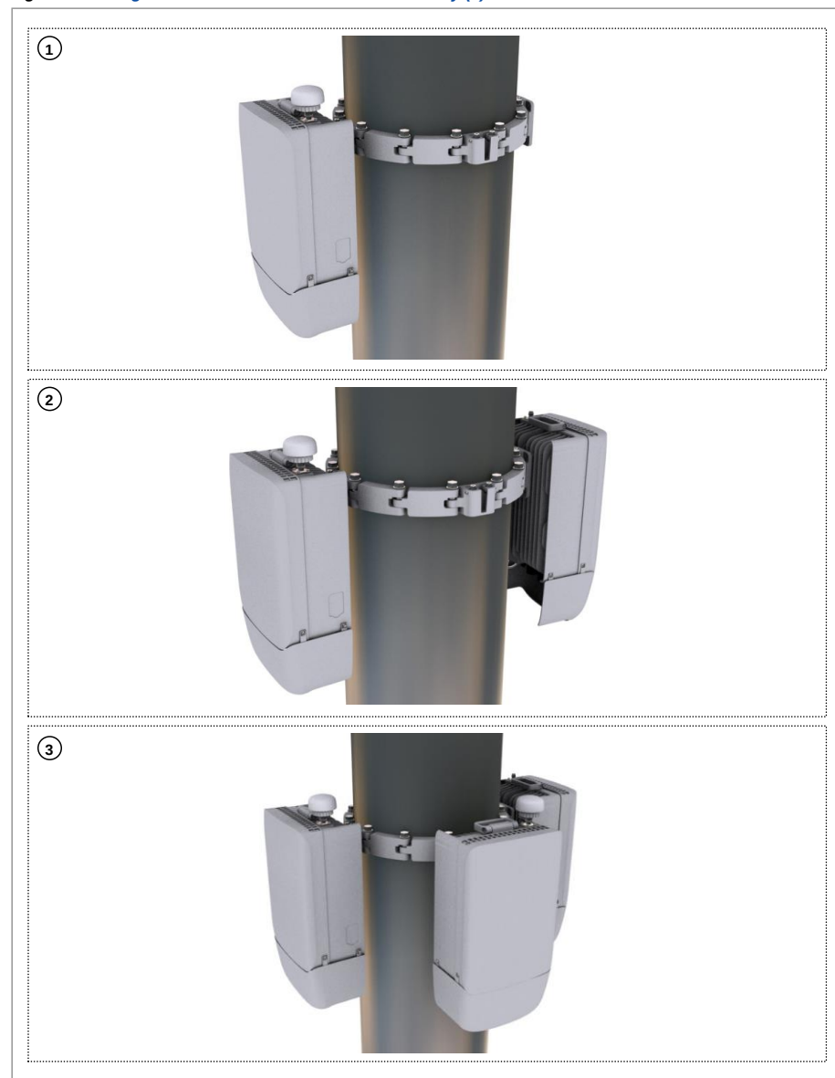
Figure 29. Fixing AU on the Pole Chain Bracket Assembly (2)
