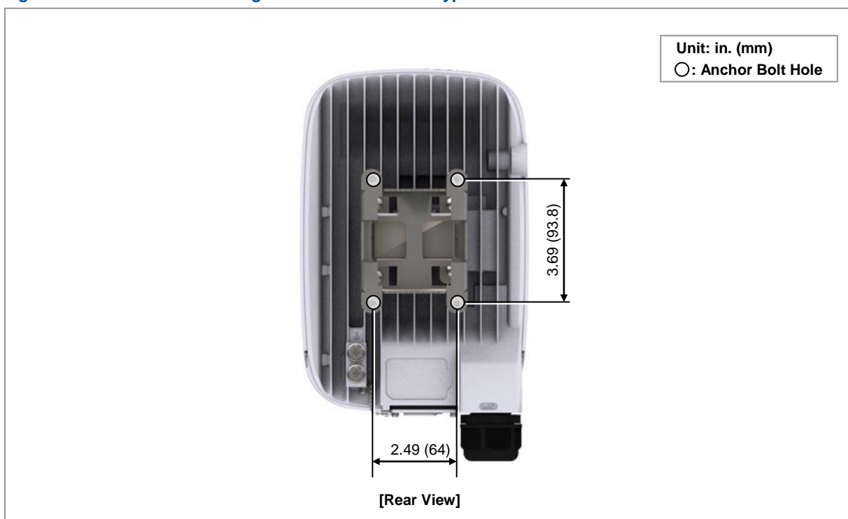
Figure 13. CPE Outdoor Marking Dimensions for Wall Type
